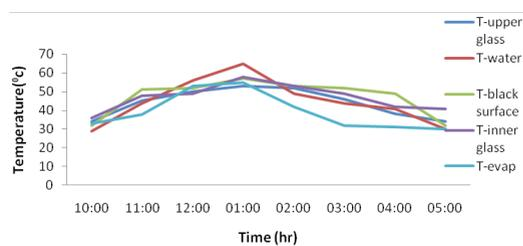
**Fig. 6: Variation of temperature with time when water level 1 cm**
