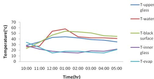
**Fig. 7: Variation of temperature with time when water level 2 cm**
