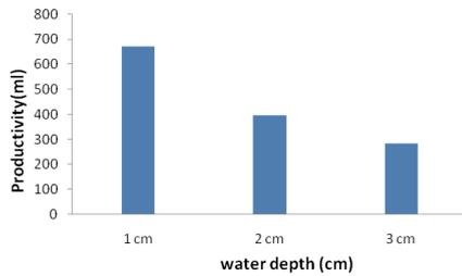
**Fig. 9: Cumulative productivity for various water depths with Passive solar still**
