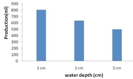
**Fig. 10: Cumulative productivity for various water depths with Active solar still**
