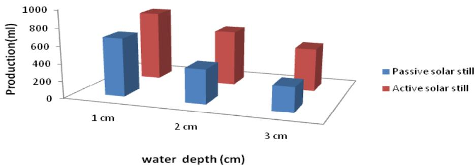
**Fig. 11: Cumulative productivity for various water depths with Active solar still**
