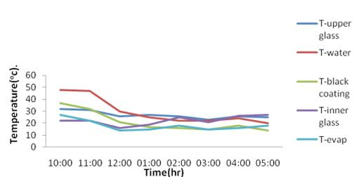
**Fig. 8: Variation of temperature with time when water level 3 cm**
