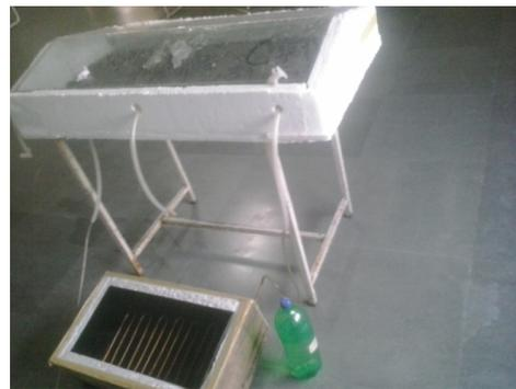
**Fig. 2: Experimental Setup of double slope glass active solar still**
