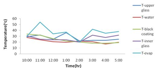
**Fig. 4: Variation of temperature with time when water level 2 cm**
